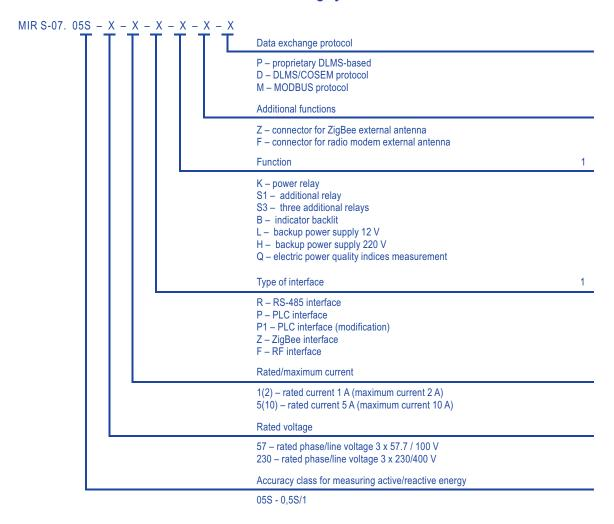
1. If there are several functions or interfaces, their codes are written sequentially, for example, a meter featuring PLC, ZigBee and radio interfaces will have a PZF code.
